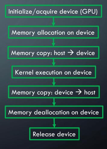
• Simple example: adding 2 arrays [from https://developer.download.nvidia.com/compute/DevZone/docs/html/C/doc/CUDA C Programming Guide.pdf]
